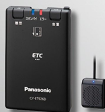
ETC [ Electronic Toll Collection system ]
